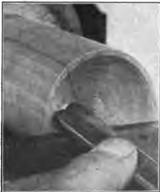
Fig. 101. Turning Inside of Box Cover.
